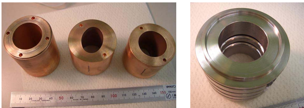
Fig. 19 Parts for the present RF load. Left: three parts for a polarizer. Right: lossy cell.
